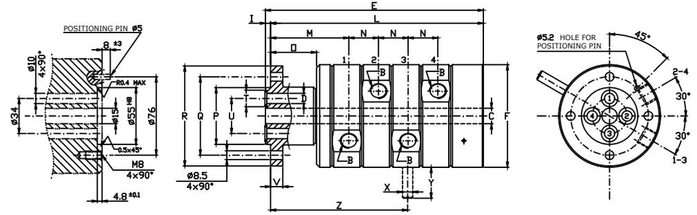
**UK ROTOFLUX TWO, FOUR, SIX PASSAGES WITH A STRAIGHT CENTRE BORE**
